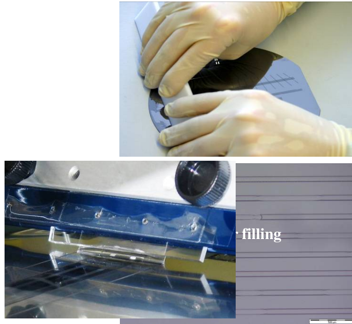
Fig. 3.19 blading step during waveguide fabrication and overfilling due to incomplete blading
